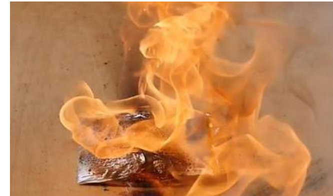
Nail penetration test in Li Ion cell
